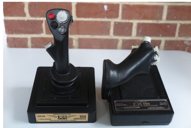
THRUSTMASTER: F22 AND TQS - THESE REFINED AND FULLY PROGRAMMABLE CONTROLLER DESIGNS ATTEMPTED TO SIMULATE THE REAL AIRCRAFT CONTROL SYSTEMS USED ON THE F-16 FIGHTING FALCON
