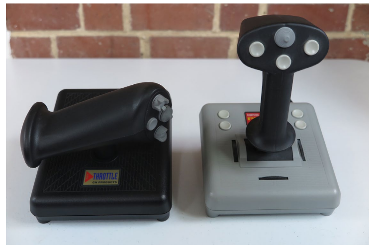
CH PRODUCTS: FLIGHTSTICK PRO & PRO THROTTLE - SEVERAL MANUFACTURERS DEVELOPED THEIR OWN LINE OF COMPETING HOTAS SYSTEMS FOLLOWING THE POPULARITY OF THRUSTMASTER'S DESIGNS; UNLIKE THE FCS/WCS COMBO, THESE ARE NOT PROGRAMMABLE
