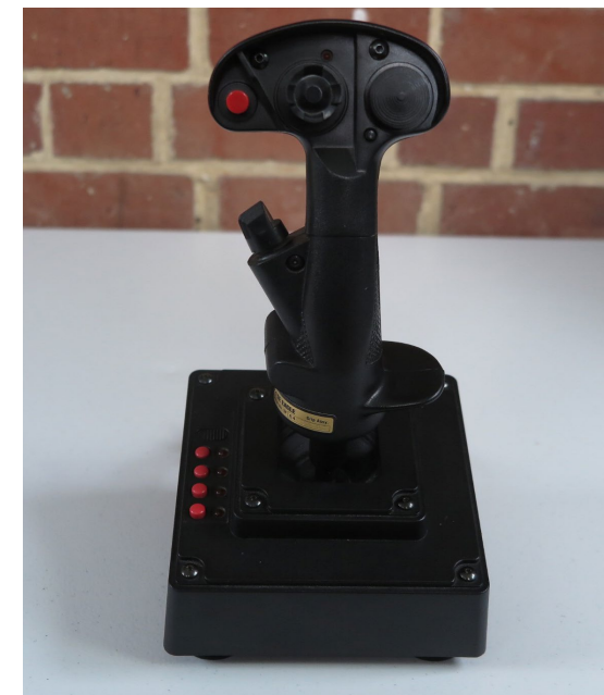
SUNCOM EAGLE (RIGHT): INSTEAD OF USING SOFTWARE TO PROGRAM BUTTONS FOR A PARTICULAR GAME THIS UNUSUAL FLIGHT STICK WAS PROGRAMMED EXTERNALLY USING AN AT KEYBOARD CONNECTION BEFORE FLIGHT
