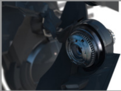
individual engines can rotate in the wing housing ENGINES
