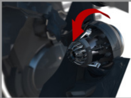
individual engines can rotate in the wing housing
